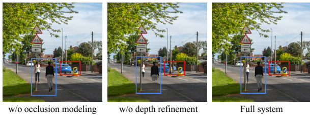
Figure 14: Monocular depth estimation could be off in shadow regions (red box) or have vague boundaries (blue box). Semantic segmentation information helps refine the depth value on grounded, thin objects.
