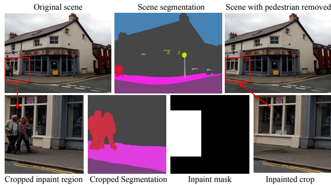
Figure 3: Stable Diffusion [Rombach et al. 2022] based inpainting. We detect existing people and cars with segmentation map, crop the surrounding region, inpaint and compose back to the image.
